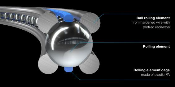
In a wire race bearing, highly resilient bearing rings made of wire assume the function of the bearing arrangement. This saves weight and space. The free choice of material and the free design of the enclosing structure also allow the weight of the overall product to be reduced considerably.
