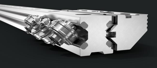
Franke linear guides are the first choice when highest dynamics are required. The large rollers are mounted very smoothly. They run with low friction and precisely guided on the inserted tough and hard steel wires. Because almost exclusively light aluminum is used for the entire construction, the moving mass is low. The result: Highest dynamics and energy efficiency.
